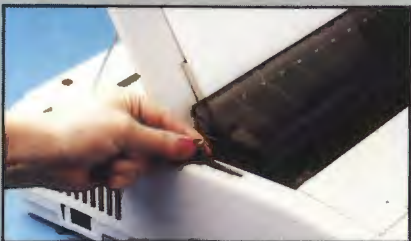
Automatic single-sheet paper feed.
