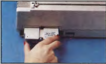
Plug-in interface cartridge enables easy connection with various computers.
